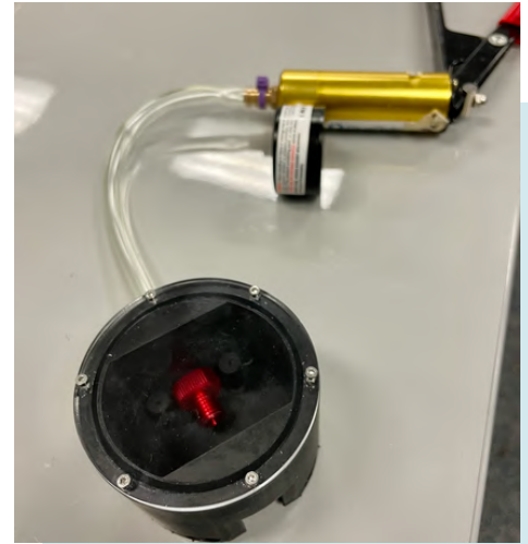
Fig 29. Vacuum testing camera enclosure
